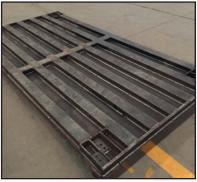
Continuous welding Multiple steel channels
