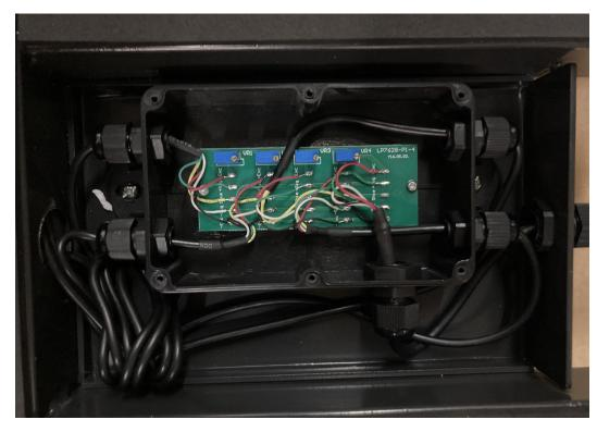
If all the wires are in place and none are loose then your scale should be fine assuming there is no damage to load cells or water in the junction box.
