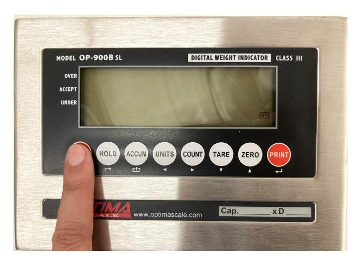
Make sure the unit is plugged in. The most common problem is a bad keypad. We will be testing if the unit is working properly by trying to turn on the unit without using the keypad.
