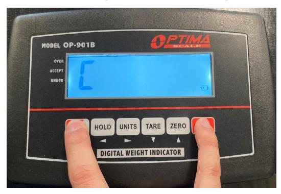
Press and hold the **ON/OFF** button and **SET** button at the same time for 3 seconds to get into calibration mode.
