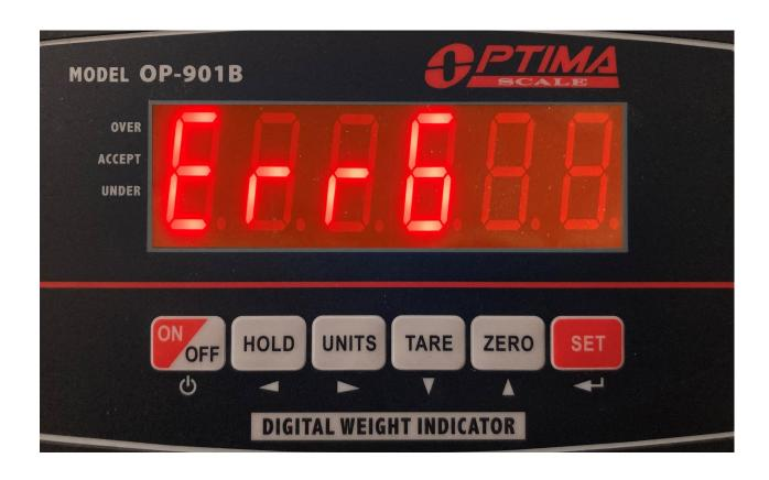
The first step would be to check the wiring.
