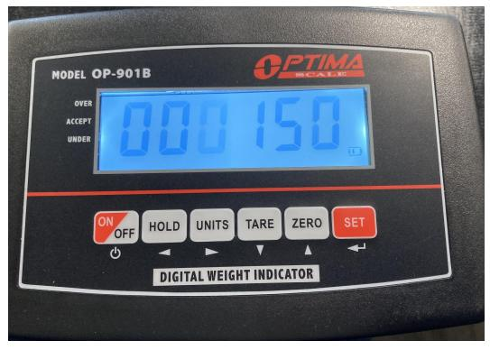
This is my correct weight of 150 lbs. Place the weight on the scale. With the weight on the scale and the matching weight on the screen press the SET button. CAL
