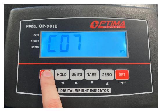
With nothing on the scale press the **ON/OFF** button. This will save all your work. You are done with calibration.
